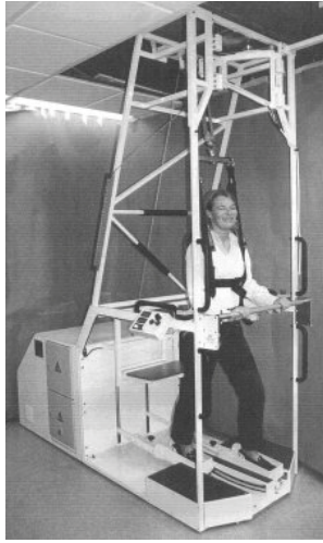
Figure 1.3: Gait Trainer I Predefined footsole-trajectory controller, with passive weigh compensation system
