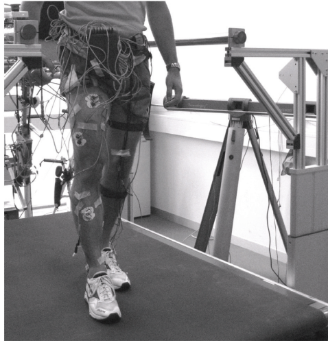
Figure 8.2: Fully equipped test subject. The left leg carries the position tracking markers, the right leg the EMG electrodes. The subject is not yet connected to the LOPES robot
