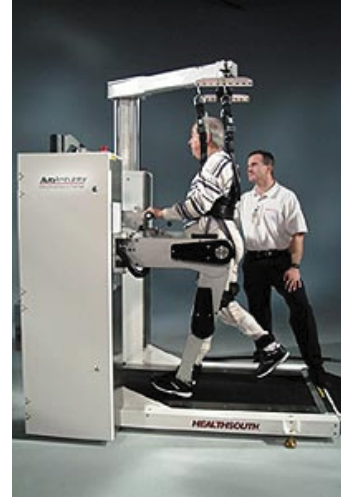
Figure 1.4: AutoAmbulator 4 DoF servo-controlled exoskeleton, with passive weigh compensation system
