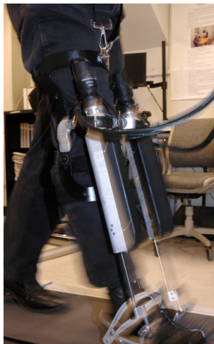
Figure 1.6: Anklebot, driven by a DC motor driven linear traction drives.
